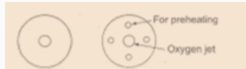
Fig- differences in torch tips for gas welding and gas cutting
