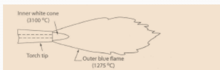
Oxy-acetylene gas welding neutral flame
